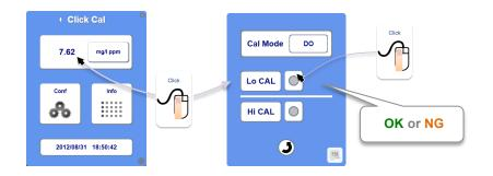
Stabilize the measurement value in a buffer, Oxygen free air and so on to receive OK.
